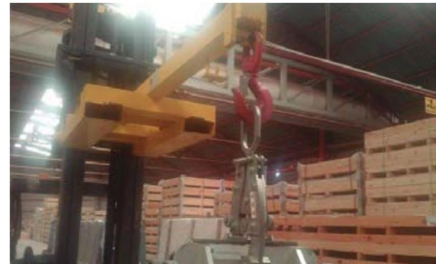
If slings are used or any other handling equipment with metallic parts, make sure that the metal does not come into contact with the surface of the slabs.
