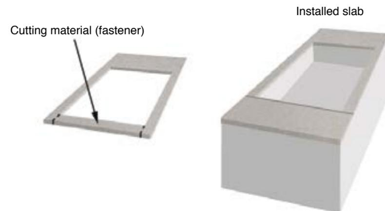
If the wrong type of cutting tool is used, the machine or slab might be damaged or even break. Problems might also occur if the whole weight of the slab is concentrated on one single point as it is cut, due to pressure from the cutting disc. For this reason, it should be cut by passing the cutting disc across it several times. Remember, too, that too slow a cutting speed can be counterproductive since the diamond edge might get damaged and the cutting disc have to be changed.
