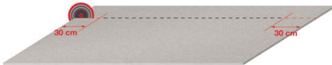
The cutting speed for 45° mitred joints should be 0.5 ml/mins.
