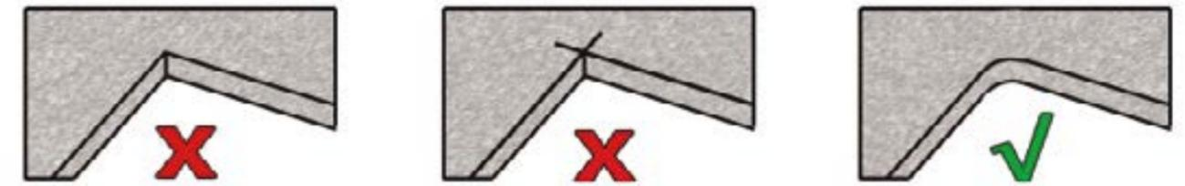
To make the corners of the cut-out, drill them with a bit with a radius of >3 mm.
