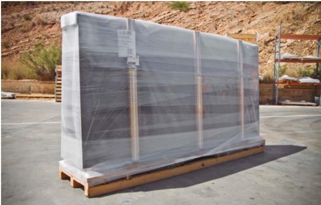
Once all 20 slabs have been packed onto a pallet on their A-frame, the corners are protected with 4 cork corner protectors. The slabs are also secured to the pallets with 3 slings, mounted on wood strips to prevent them from coming into direct contact with the slabs. The pallet is then secured with plastic straps to protect it from the rain and the elements.
