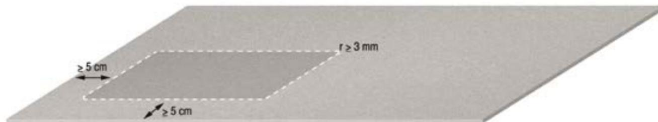
A bigger radius will ensure a higher structural resistance. In contrast, angles with no radius create a stress point on the surface. NEVER LEAVE 90° ANGLES.
