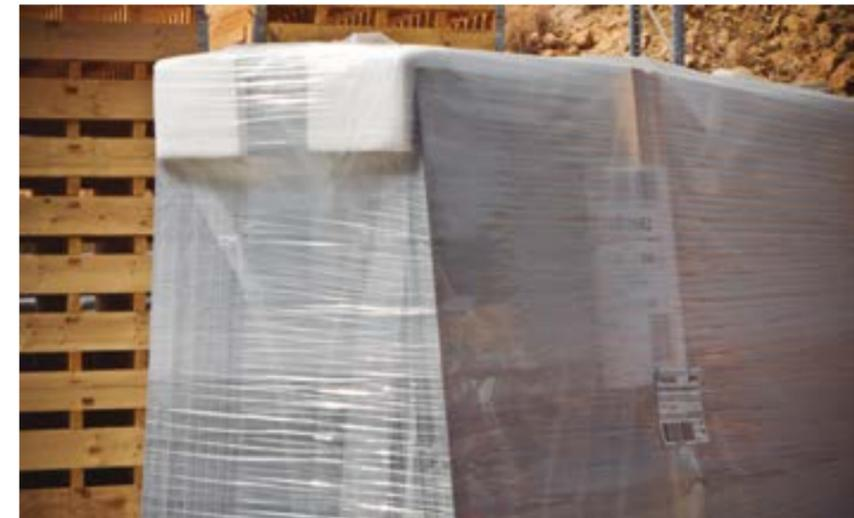
Each A-frame bears a label with the name of the series, colour, finish and shade of the product, together with the batch number and quality rating to ensure its full identification. The label also lists packing details such as the weight, m<sup>2</sup> per A-frame and number of slabs per A-frame.
