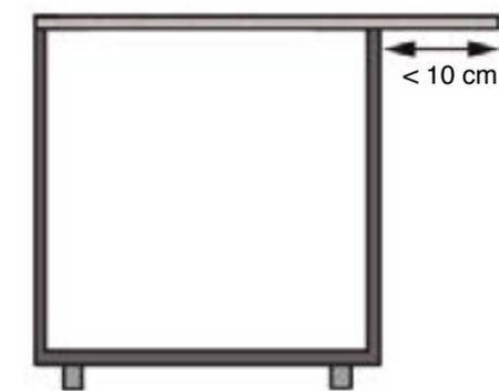
If there is room and you would like it to jut out more, a prior study must be made of the necessary reinforcements to use in each particular case.
